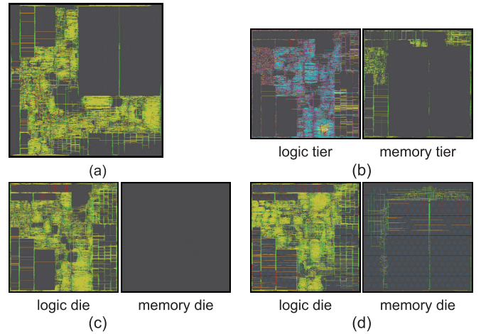
Fig. 12. Clock tree layouts in our 2-D and heterogeneous 3-D designs. (a) 2-D. (b) M3D. (c) Hybrid bonding 3-D. (d) Microbumping 3-D.
