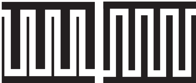
Fig. 4. A test structure pair that can distinguish between the impact of density and linewidth (top view).
