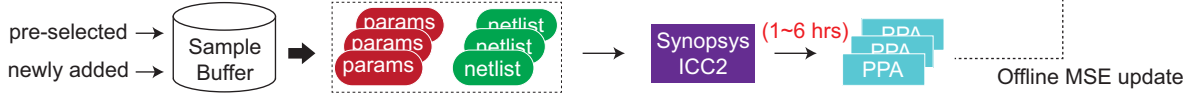
Figure 1: High-level overview of our hybrid framework. FastTuner optimizes parameters sequentially online by leveraging the pre-trained offline PPA estimator to provide reward feedback, preventing the need for time-consuming ICC2 feedback.
